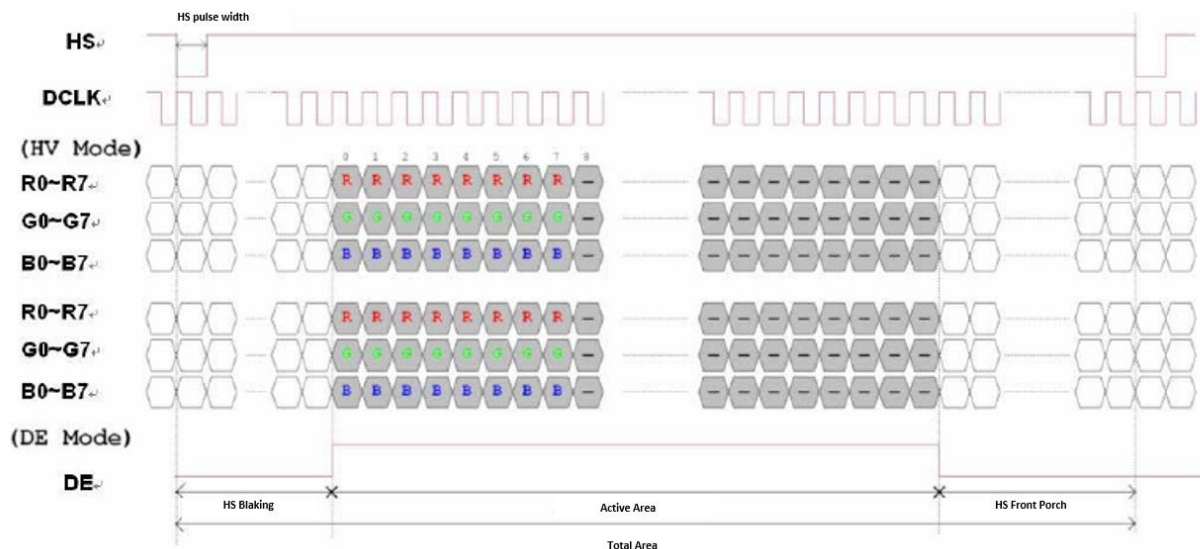
Figure 9. Horizontal input timing diagram
